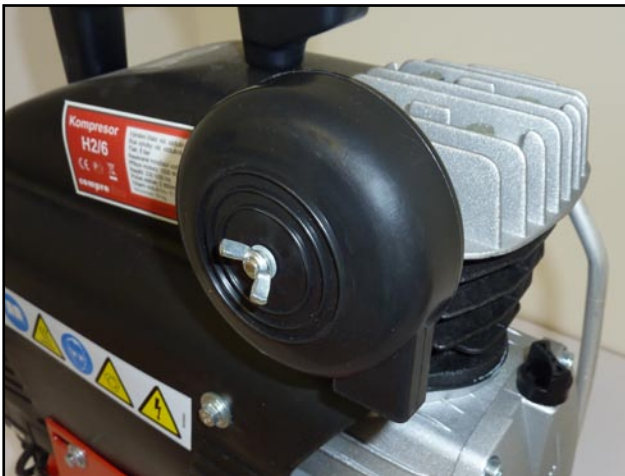
Photo of suction filter screwed onto compressor
