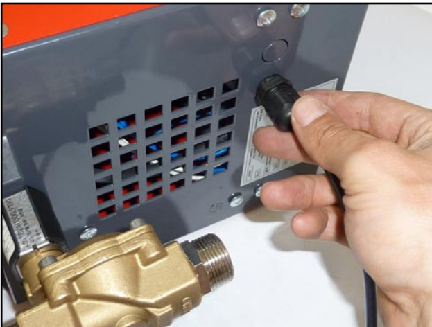
Pull the solenoid connecting cable using the grommet through the cut out hole in the lower part of the burner body
