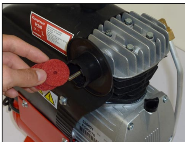
Cleaning compressor filter
