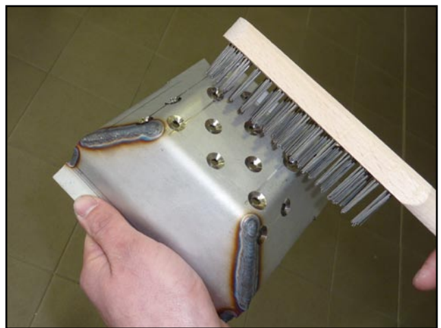
Example of cleaning the combustion chamber
