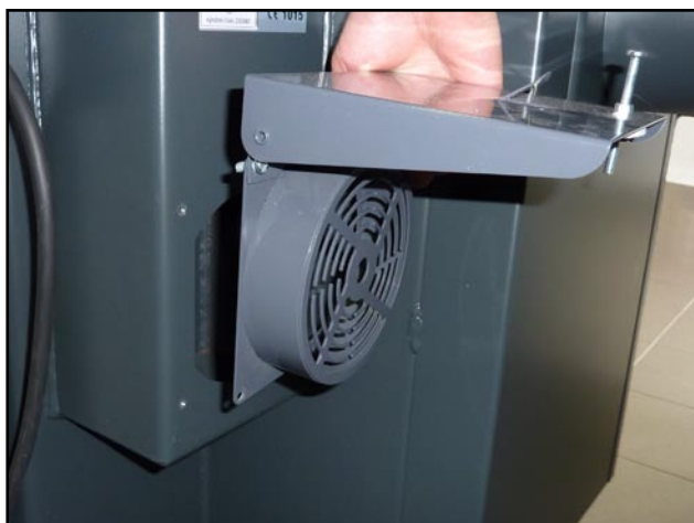
Disassembling flap for combustion air inflow
