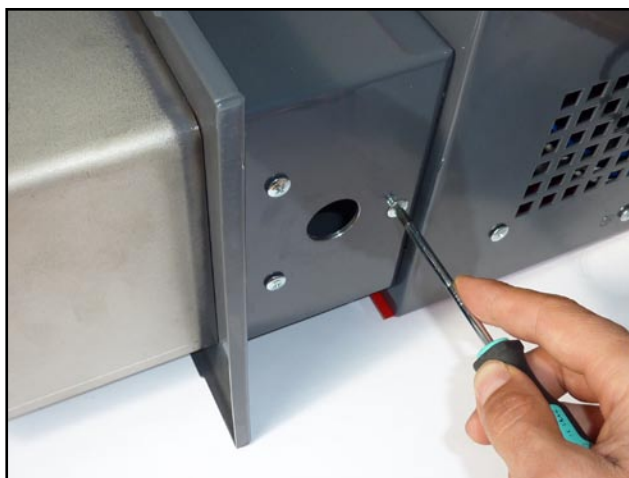
Screw the original screws back into the holes so air cannot flow through them or false air be sucked through them
