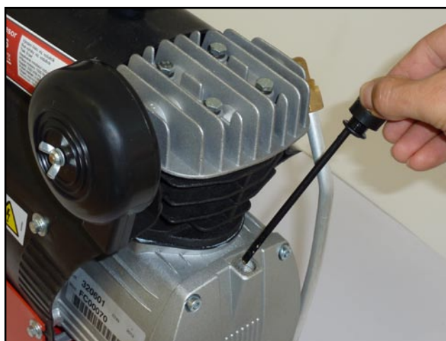
Checking oil levels in compressor
