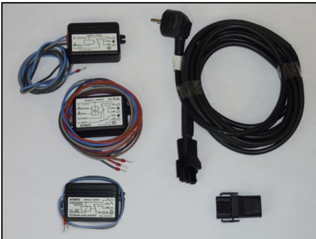
AD02, AD03 and AD04 modules Connecting cable with 3-pin connector (female) and separate 3-pin connector (male)
