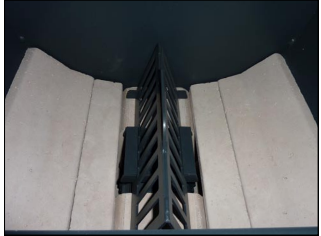
Positioning special grille for gasifier nozzle for DCxxRS boiler
