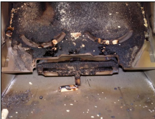
Slight clogging after 4 months of use
