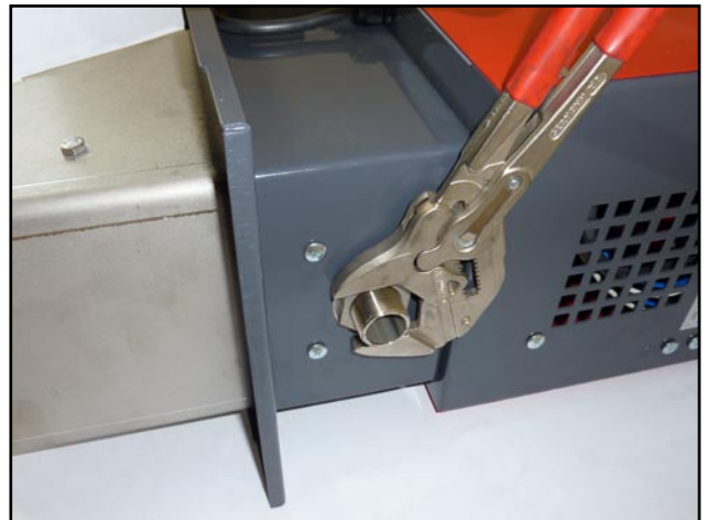
Carefully tighten the nuts with washers to the burner body
