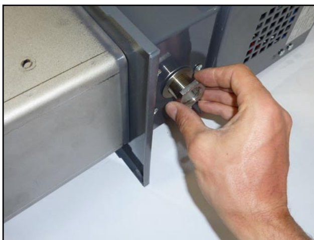
Set the pneumatic cleaning channel in the burner and gently secure using washer and low nut
